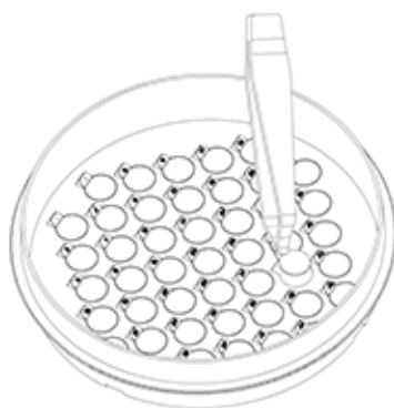
Step 2: Pull apart the break point of cell slide in the horizontal direction
