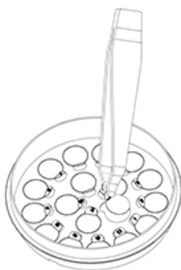
Step 2: Pull apart the break point of cell slide in the horizontal direction
