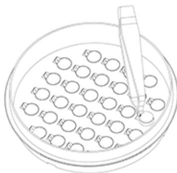
Step 2: Pull apart the break point of cell slide in the horizontal direction
